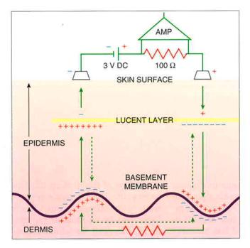
If current is allowed to flow from the positive side of a source back to the negative side through electrodes on the skin surface, the lucent layer and basement membrane act as capacitors. Charging these capacitors generates a potential gradient that counteracts the current flow.
